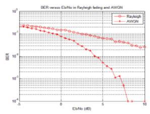
Fig. 2. BER in Rayleigh fading and AWGN.
